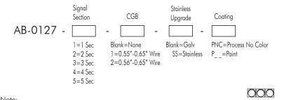
Stainless upgrade includes stainless steel fasteners and pins on span wire clamp.
