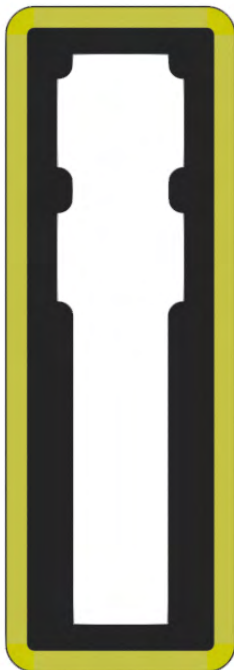
BK-1014-RT2 SERIES 12"-12"-8"-8"-8", 5-Section w/ Reflective Tape EXAMPLE
