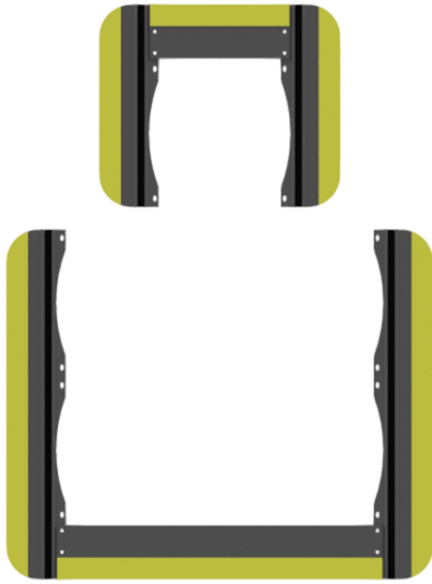
BK-8105-17-RT2-EagleSG-FL-PNC 12", 5-Section Cluster Eagle SG, 17" CTC w/ 2" Reflective Tape EXAMPLE
