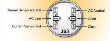
Diagrams are shown looking into the wired meter base.
