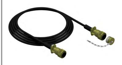
7-conductor 12 AWG cable x 35' long with female Mil-Spec connectors both ends and protective cap one end. For connecting junction box to meter.
