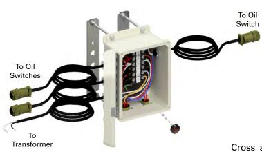
Cross arm mount. Supplied with a 6-circuit terminal strip, oil switch cables, and transformer cable. Includes Mil-Spec connectors for sensor cable and meter base.
