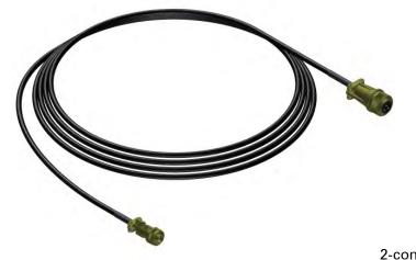
2-conductor 16 AWG cable x 25'-0" long with male and female Mil-Spec connectors. For use with Lindsey Sensor and Junction Box wired for Lindsey or Fisher Pierce Sensors.
