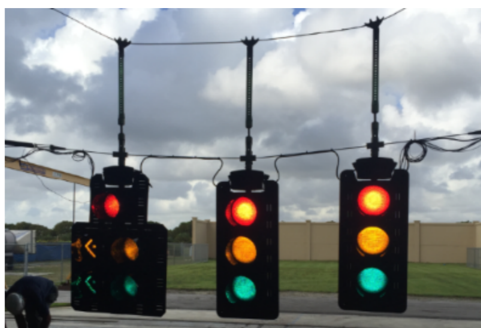
*Cable concept tested in 150 MPH winds at the FIU Wall of Wind supporting a traffic signal with NO failures.
